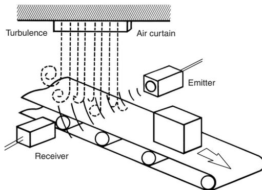
The jetting sound of air nozzles includes noise of a wide frequency range, which will affect the operation of the E4B. Do not use an air nozzle near the E4B.
