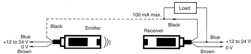
**Note:** Be sure not to make mistakes in polarity when connecting the above wires. In other words, both brown lead wires must connect to +DCV or 0 V and both blue lead wires must connect to 0 V or +DCV. Otherwise, the indicator of the Emitter will be lit when the ultrasonic beam is interrupted.
