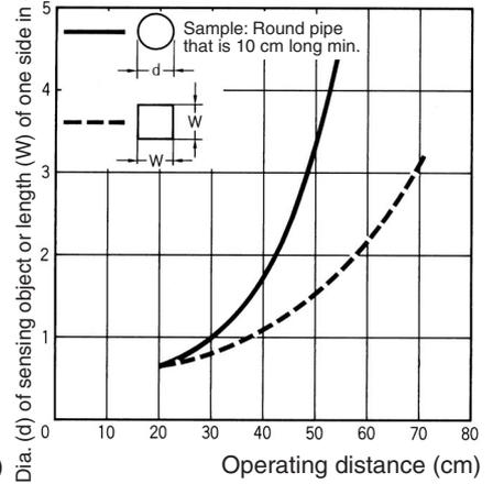
**Note:** The curve with the sensitivity adjuster set to maximum indicates the size of the sensing object.
