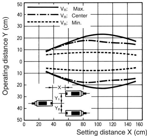
**Note:** Obtain the point that turns  $Y_1$  and  $Y_2$  ON while changing the sensing distance (X).
