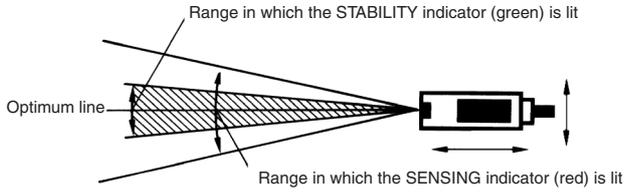
Pass the sensing object through the sensing range and adjust the sensitivity so that the SENSING indicator turns ON and OFF according to the presence or absence of the sensing object while the STABILITY indicator is lit continuously.
